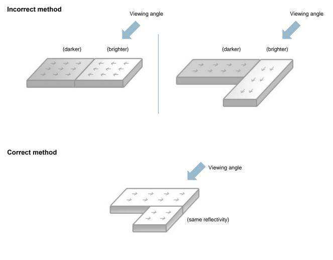
The variation of the particulate distribution pattern between two separate pieces seamed together may be obvious and easy to notice if not fabricated as suggested in this technical bulletin. On your Pearl particulates project we strongly suggest that you experiment, prior to actual fabrication, with the methods and procedures described above.
