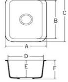
Α 12.83in (326mm) В 14.01in (356mm) С 16.37in (416mm) D 10.47in (266mm) Е 6.49in (165mm) F 7.08in (180mm)
