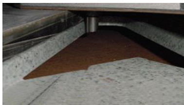
(3) Rout with 12mm( \frac{1}{2} " ) straight bit 25mm(1" ) guide
