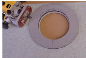
(2) Rout out damage with 12mm(1/2") straight bit 25mm(1") template guide [ 24.3 - A ]
