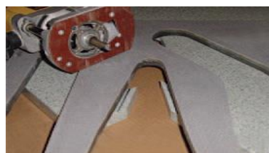
(8) Rout out cracked build up
