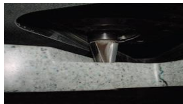
(4) Rout bevel into counter
