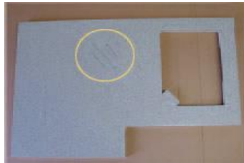
(1) Hot pot cracks
