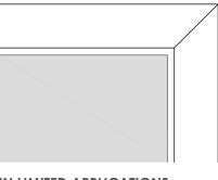
IN LIMITED APPLICATIONS FABRICATORS MAY OPT FOR A MITRE JOIN WHEN USING HEAVILY PATTERNED DESIGNS.
